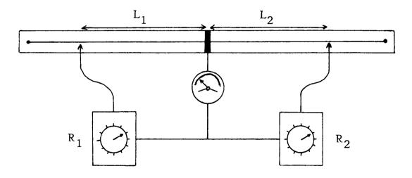
The subjects' task was to balance the arrangement (bring the needle on the meter to zero) by altering  $L_1$ ,  $R_1$ ,  $L_2$  and  $R_2$ , the way in which these variables could be altered was demonstrated to the subjects before they started playing with the system. The balance position for the set-up occured when:
