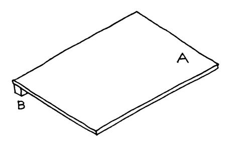
The desired angle can be obtained by placing or fixing a piece of wood under the top edge.
